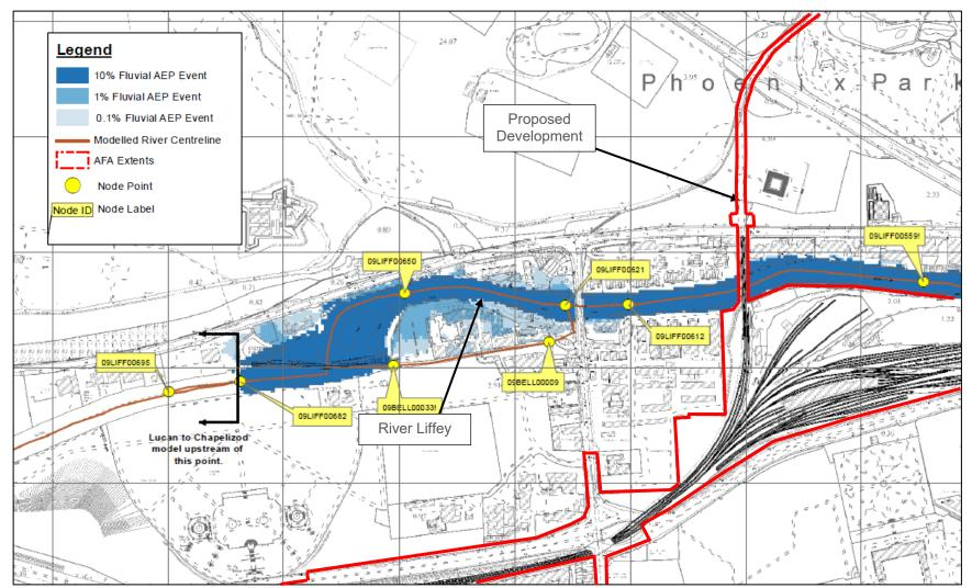
Figure 5-15 Eastern CFRAM Study - Liffey fluvial flood extent map (1) <sup>10</sup>
