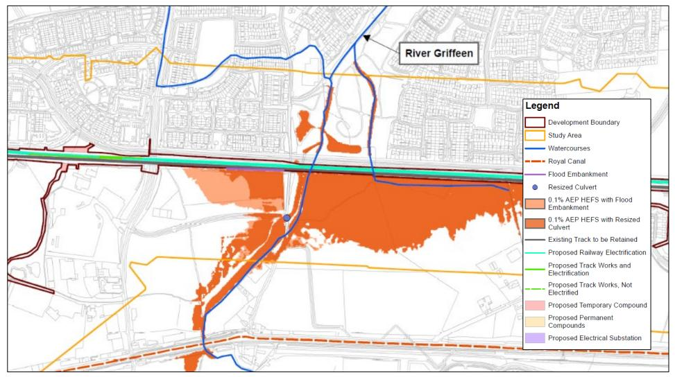
Figure 3-45 Flood extents for the Lucan and Griffeen Streams with proposed mitigation measures in place
