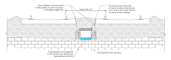
Figure 6-3 Typical section on Phoenix Park Tunnel showing existing drainage. Source: Phoenix Park Tunnel, drawing SDS-15-152-P03-022
