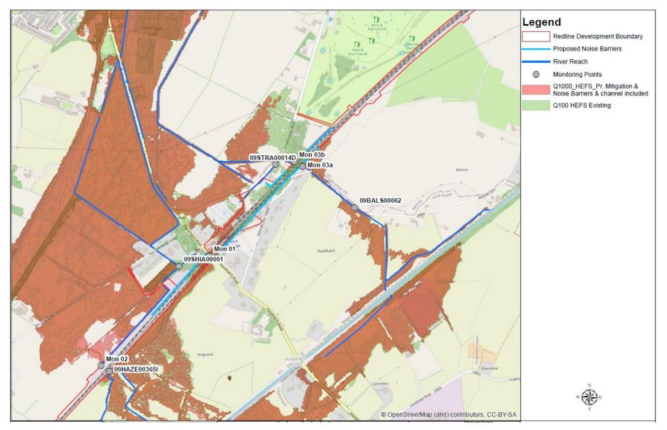
Figure 3 20 Comparison of 0.1% AEP HEFS flooding extents for existing and proposed scenarios (with mitigation measures)
