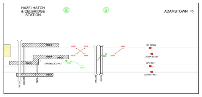
Figure 3-2 Hazelhatch & Celbridge Station – Schematic Track Plan (in red trackwork within this project)
