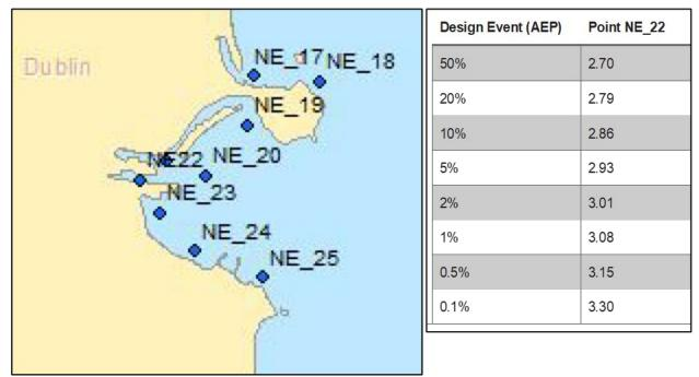
Figure 5-10 ICPSS - Overview of Surge Model Runs, North East Coast – ICWWS - Water Levels for NE\_22 – Meters to OD Malin (OSGM-15)
