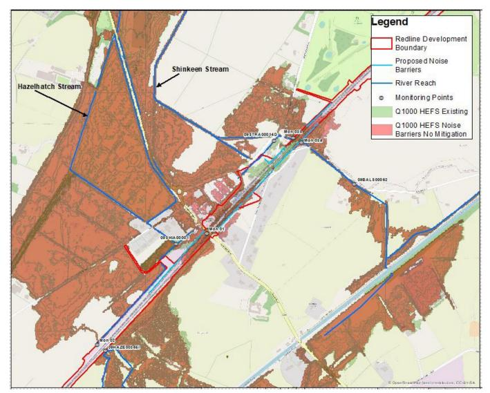
Figure 3-19a Comparison of 0.1% AEP HEFS flooding extents for existing and proposed scenarios (with noise barriers)
