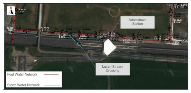
Figure 3-22 IW GIS Database – Storm and Foul Network in the vicinity of Lucan Stream Crossing the Railway
