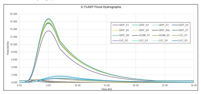
Figure 3-39 Design Flood Hydrographs for 0.1% AEP
