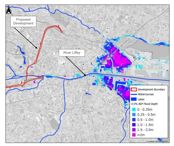
Figure 5-14 Extract of National Coastal Flood Hazard Mapping 2021 Depth map at 0.5% AEP (1 in 200 chance in any given year) (Source: OPW)
