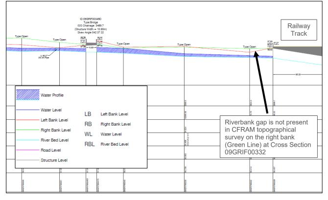
Figure 3-42 Longitudinal profile of the Griffeen River upstream of the railway
