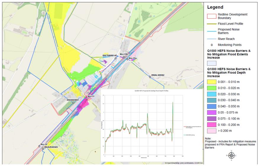
Figure 3-19b 0.1% AEP HEFS Flood profile through agricultural land downstream of the station showing increased flooding depth for the proposed scenario (with noise barriers)
