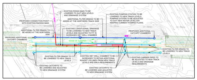
Figure 6-10 Proposed Drainage Upgrade Between OB08 and OB09
