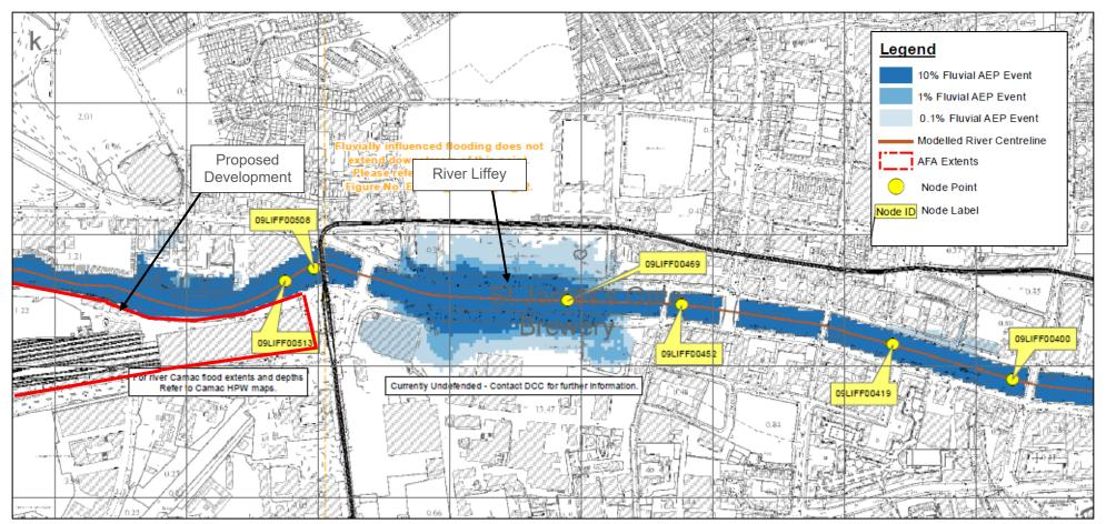
Figure 5-16 Eastern CFRAM Study - Liffey fluvial flood extent map (2)
