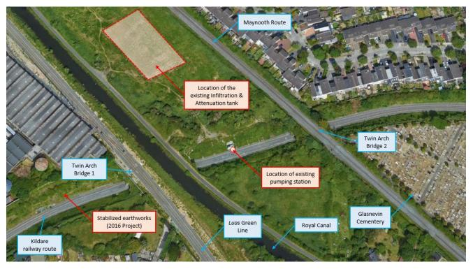
Figure 6-5 Location of the Twin Arch Bridges (OBO8 & OBO9) and existing drainage systems in the vicinity of Royal Canal.
