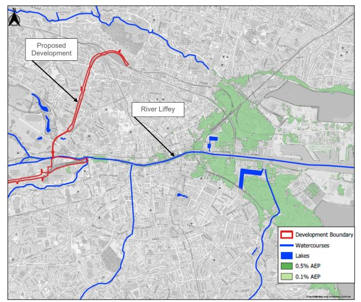
Figure 5-12 Extract of National Coastal Flood Hazard Mapping 2021 Current Scenario Coastal Flood Extent Map (Source: OPW)
