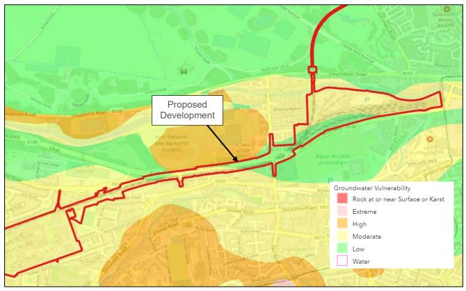
Figure 5-6 GSI Aquifer Vulnerability Mapping (Source Data and maps - GSI https://www.gsi.ie)
