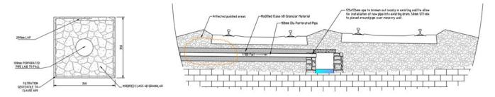
Figure 6-4 Typical section on Phoenix Park Tunnel showing existing drainage. Source: Phoenix Park Tunnel, drawing SDS-15-152-P03-023
