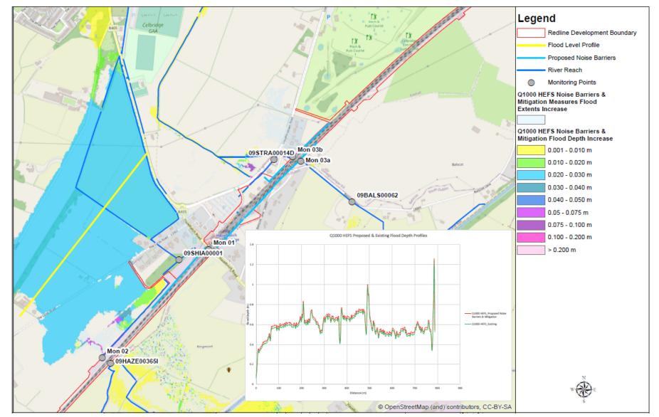
Figure 3 21 0.1% AEP HEFS Flood profile through agricultural land downstream of the station showing increased flooding depth for the proposed scenario (with mitigation measures)
