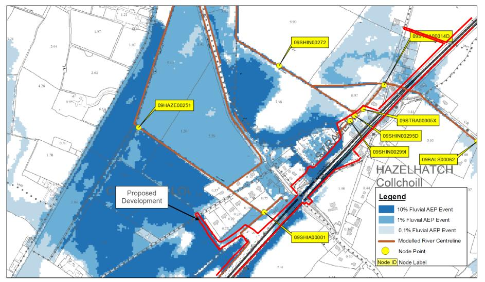
Figure 3-14 Hazelhatch Further Study (1) –MRFS Fluvial Flood Extent<sup>6</sup>
