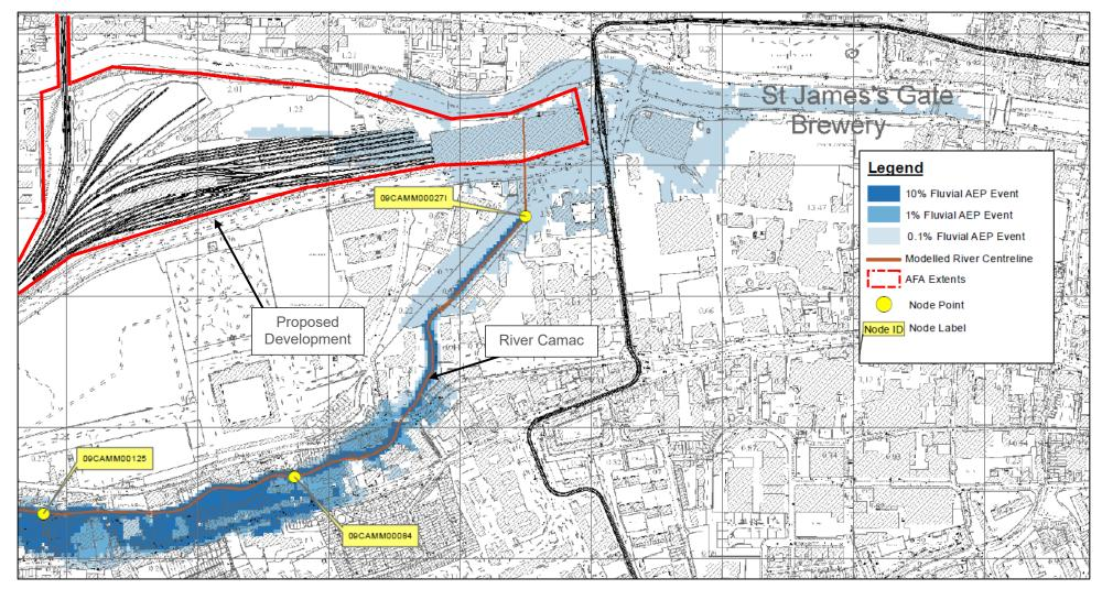
Figure 5-17 Eastern CFRAM Study - Camac fluvial flood extent map
