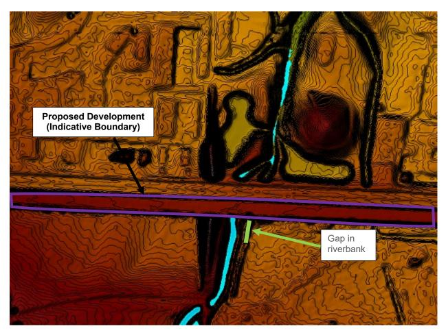
Figure 3-41 LiDAR surface for Adamstown FRA with a gap highlighted on the right riverbank
