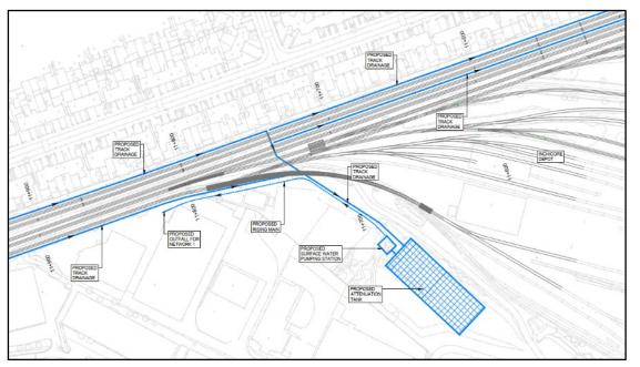
Figure 4-9 Network 1 Location of Underground Attenuation Tank
