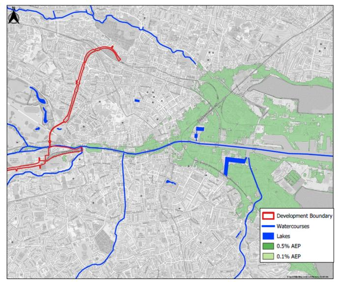
Figure 5-13 Extract of National Coastal Flood Hazard Mapping 2021 MRFS Coastal Flood Extent Map (Source: OPW)
