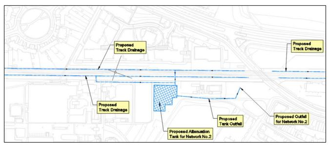
Figure 4-10 Network 2 Location of Underground Attenuation Tank
