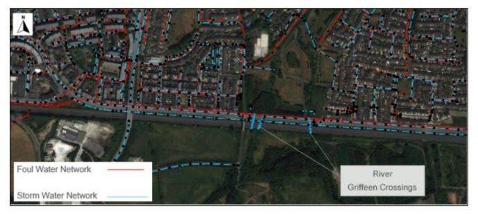
Figure 3-23 IW GIS Database – Storm and Foul Network in the vicinity of River Griffeen Crossing the Railway
