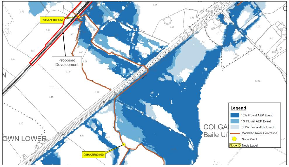
Figure 3-13 Hazelhatch Further Study (2) –Current Fluvial Flood Extent
