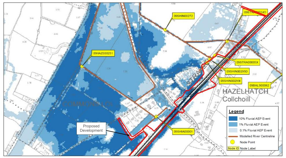
Figure 3-12 Hazelhatch Further Study (1) –Current Fluvial Flood Extent<sup>5</sup>
