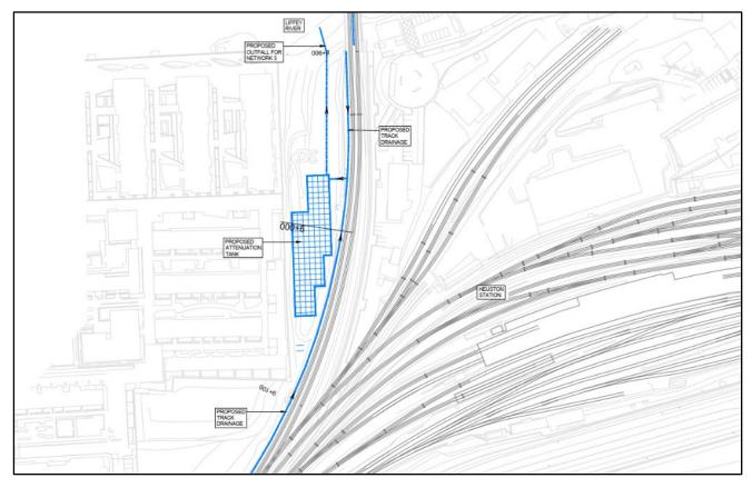
Figure 4-11 Network 3 Location of Underground Attenuation Tank
