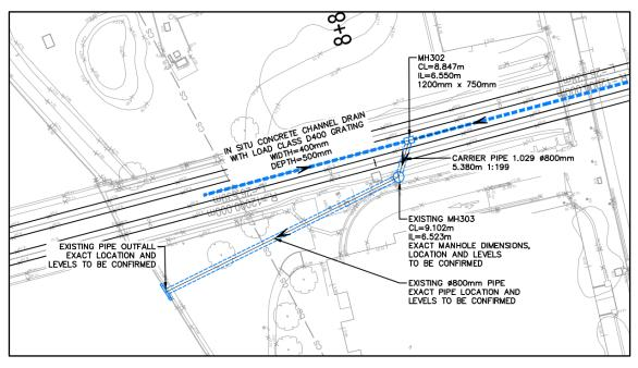
Figure 6-9 Proposed drainage works at Liffey River outfall
