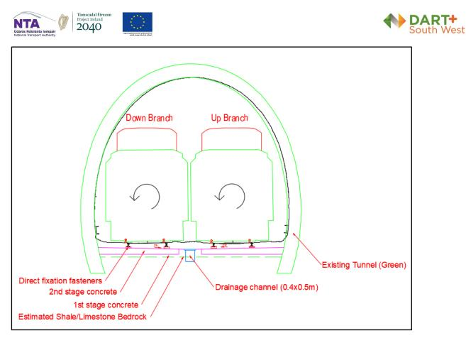
Figure 6-8 Proposed cross drainage system at Phoenix Park Tunnel
