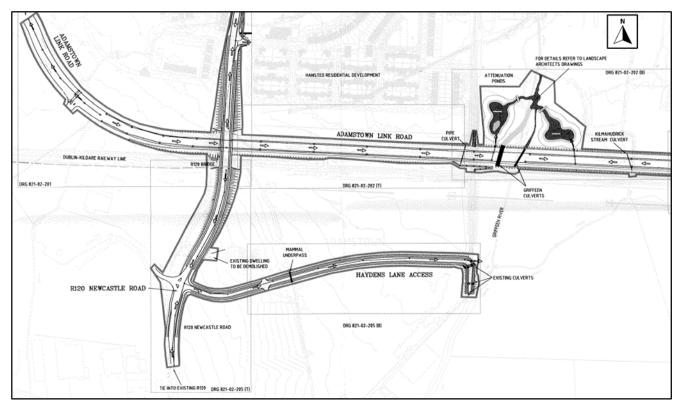
Figure 3-29 Overall Drainage Layout - Adamstown Link Road Scheme
